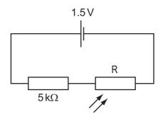
The light-dependent resistor is illuminated (in an otherwise dark room) by a flashing light.
